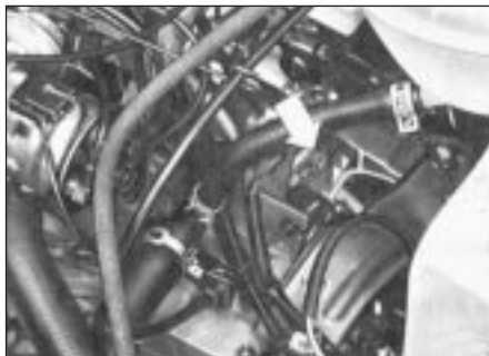
22.4 Gearbox filler/level plug location (arrowed) - 084 gearbox
