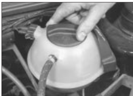
2.2 Removing expansion tank cap
