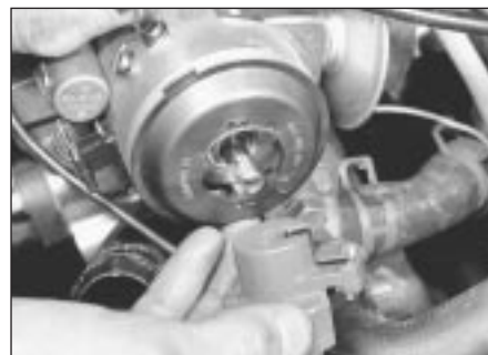
11.3 Pull off the rotor arm
