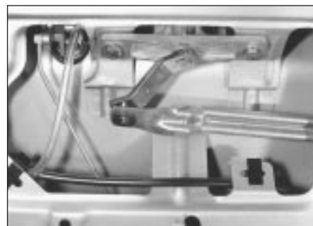
28.4a Rear wiper bearing mounting and connecting rod
