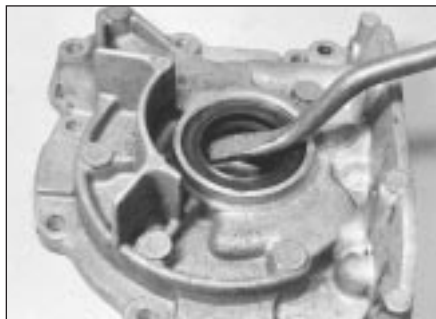
31.1 Prising out oil pump oil seal
