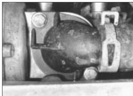
5.11a Undo the retaining bolts . . .
