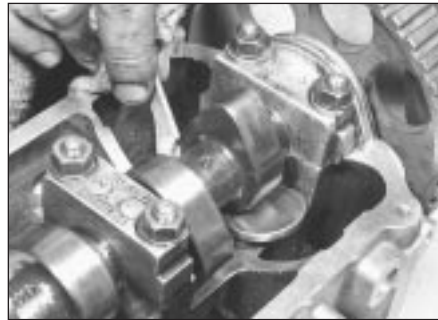
12.12 Removing a tappet bucket shim - 1.6 and 1.8 litre
