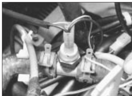
7.11 Temperature sender unit thermo-switch location - 1.05 and 1.3 litre
