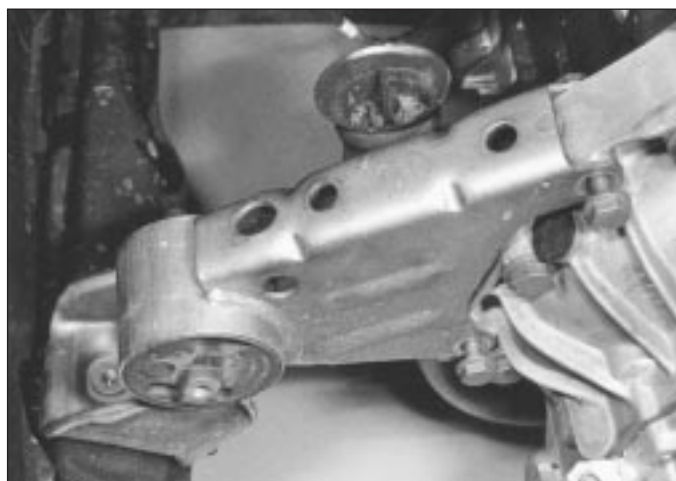
5.26b Unbolt and remove mounting unit
