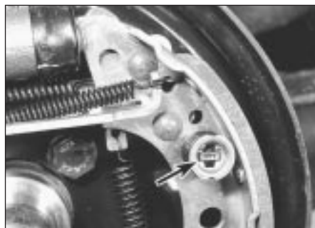
6.8 Brake shoe steady spring and cup (arrowed)
