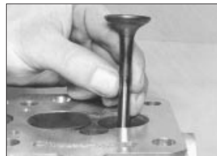
5.12 Removing a valve
