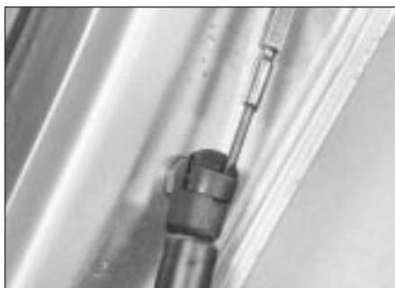
9.2a Releasing tailgate strut balljoint clip
