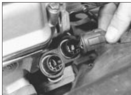
11.23b Coolant temperature switch/sender electrical connection
