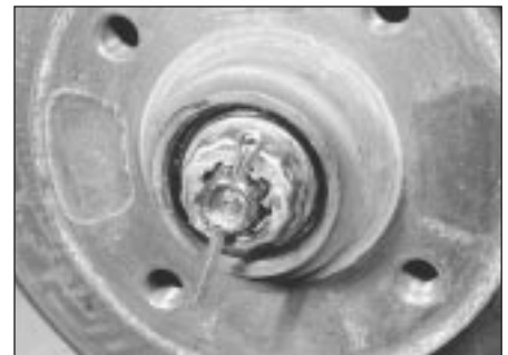
4.14 ... remove the split pin and lock ring ...
