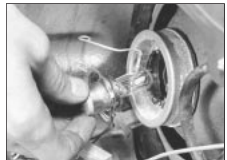
4.4 . . . and withdraw headlamp bulb
