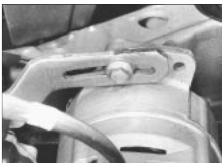
13.4a Alternator drivebelt tensioner link - 1.3 litre
