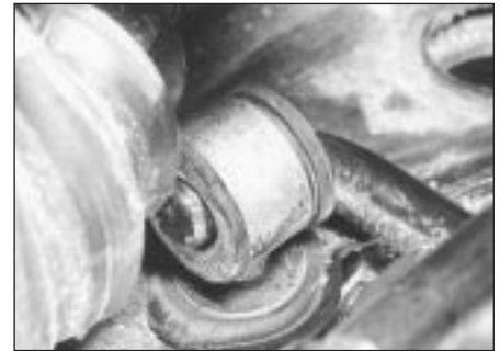
4.5 Anti-roll bar location in eye bolt
