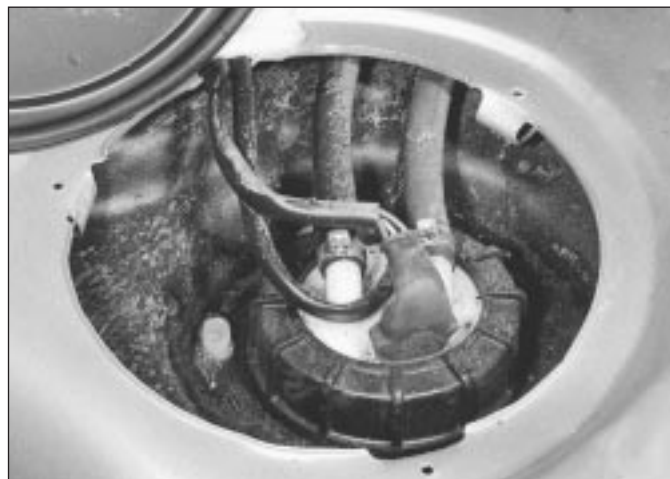
18.2 Fuel tank sender unit and connections
