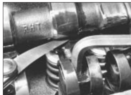
12.4 Adjusting a valve clearance - 1.05 and 1.3 litre
