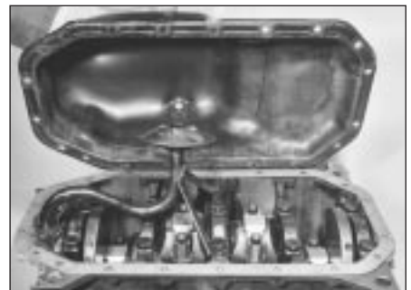
15.2 Removing the sump
