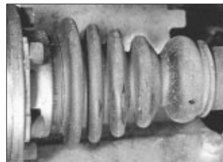
24.2 Inspect condition of each CV joint boot
