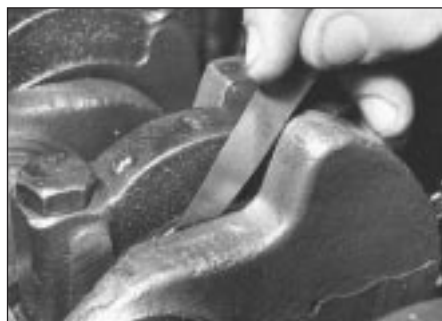
15.3 Checking crankshaft endfloat at No. 3 main bearing
