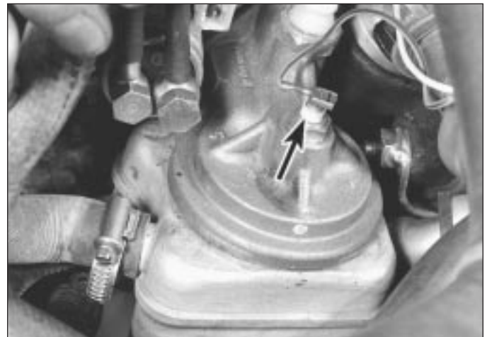
5.39 Oil temperature sender (arrowed)
