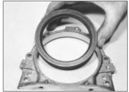
14.14 Remove crankshaft rear oil seal from housing
