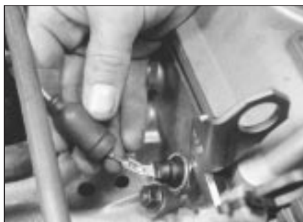
11.23c Oil pressure switch electrical connection
