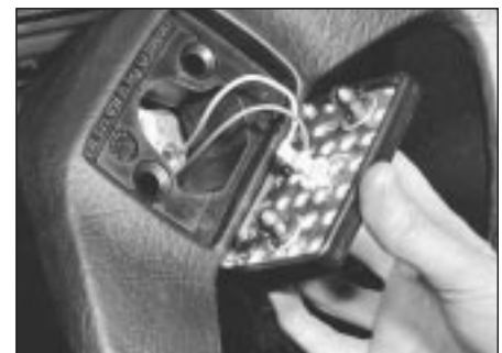
11.3a Removing steering wheel centre cover - 1.3 litre
