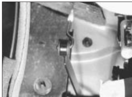
10.5 Accelerator cable-to-pedal attachment
