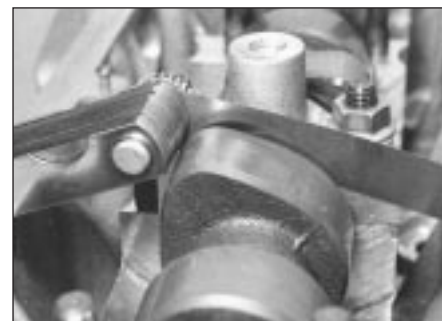
8.6 Measuring camshaft endfloat
