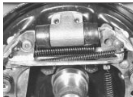
6.11 Wheel cylinder, upper return spring and pushrod assembly
