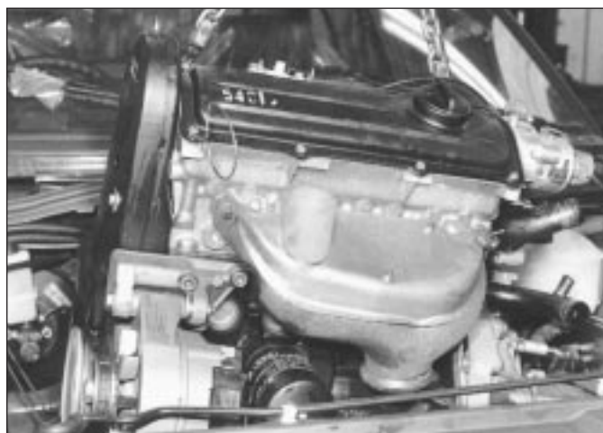
5.28 Lifting out engine/gearbox unit
