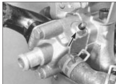
7.12 Temperature sensor (arrowed) - 1.05 and 1.3 litre
