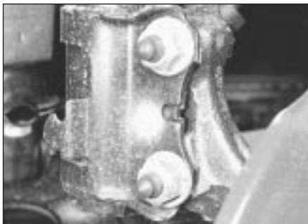
2.7 Strut-to-front wheel bearing housing retaining nuts/bolts
