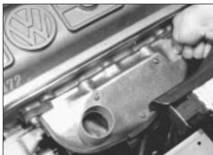
11.20 Fitting hot air shroud
