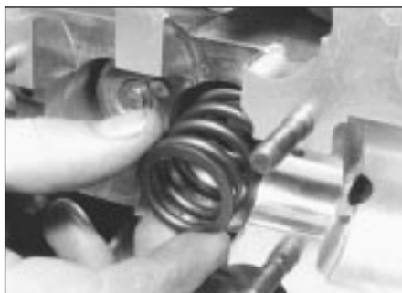
5.11a Removing an outer valve spring
