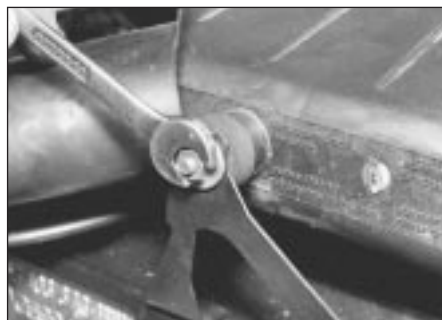
32.4b ... loosen front mounting nut ...
