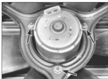
4.4 Cooling fan motor retaining nuts (arrowed)
