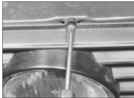
8.2 Undoing front grille retaining screws
