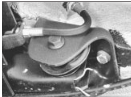
9.7 Axle beam pivot bolt head fitting position
