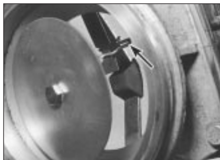
14.6 Airflow sensor plate adjustment clip (arrowed)
