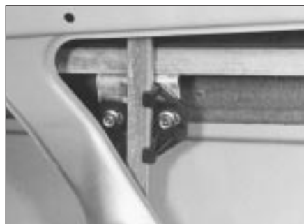
20.3b Lifting plate-to-window channel bolts
