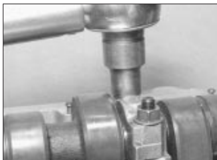
10.5 Tightening a camshaft bearing cap nut
