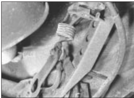
9.3 Brake pressure regulator unit showing spring bracket
