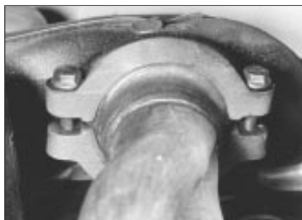
19.10 Exhaust downpipe-to-manifold flange connection - 1.3 litre
