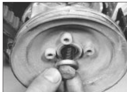
12.7 Removing crankshaft sprocket bolt and washer
