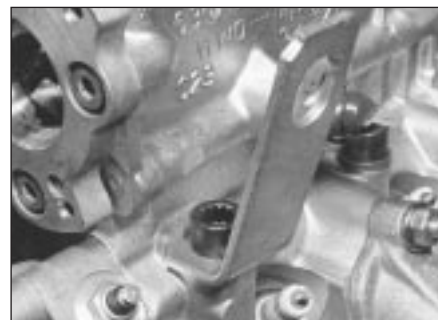
5.23 Engine lifting eye
