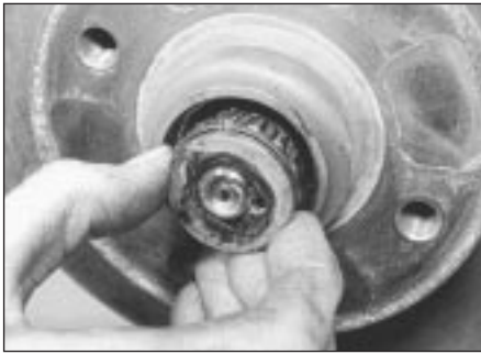
4.15 ... followed by the outer washer and bearing
