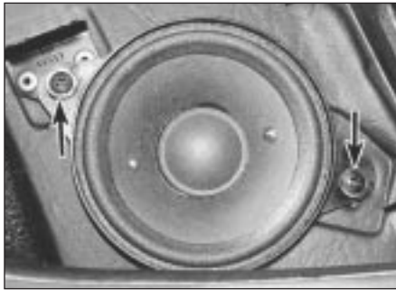
32.3 Facia-mounted loudspeaker retaining screws (arrowed)
