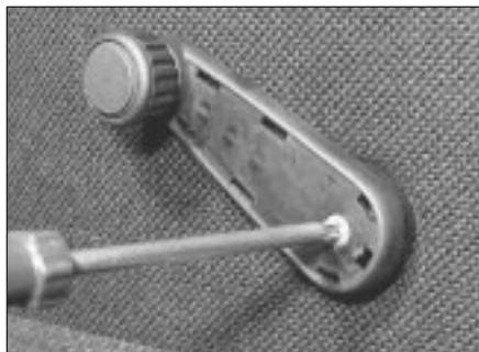
14.4b . . . and handle retaining screw
