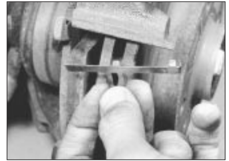
2.5 Removing a pad retaining spring
