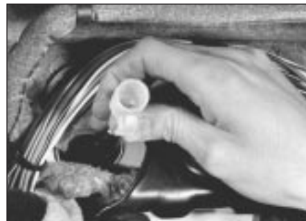
16.4 Disconnect speedometer cable
