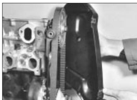
9.4 Removing timing cover
