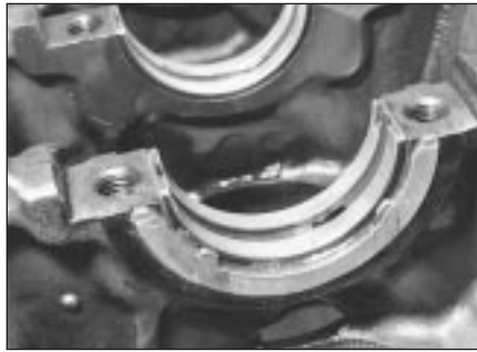
29.3 Thrustwasher location on centre main bearing
