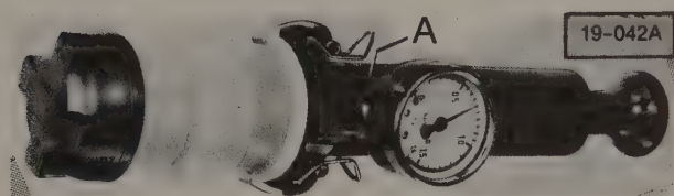
Fig. 3-1. Expansion tank cap installed on pressure tester pump (A) using adapter US 4467. Adapter is also used to pressure test the cooling system.
