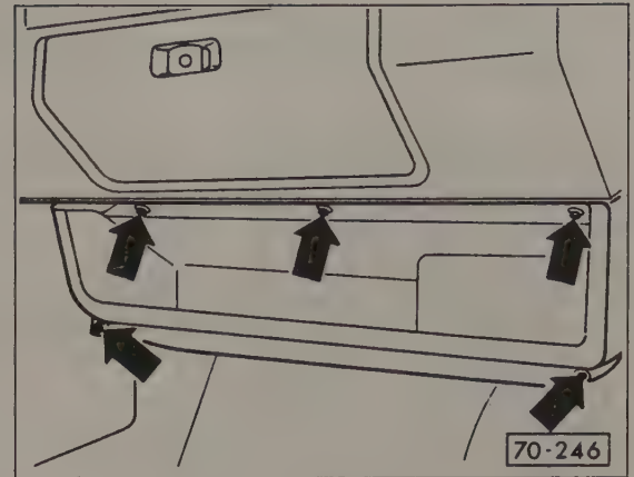
Fig. 4-8. Retaining screws (arrows) to be removed from right-lower instrument panel tray.
