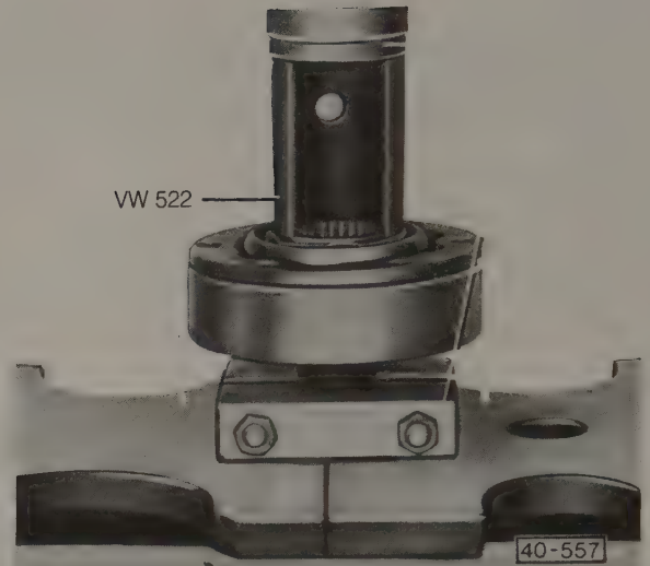
Fig. 5-11. Pressing inner CV joint onto drive axle shaft. Press tool shown, Volkswagen special tool no. VW 522 (order no. TV0 522 000 00 ZEL), allows installation of circlip while CV joint and washer are being pressed.
