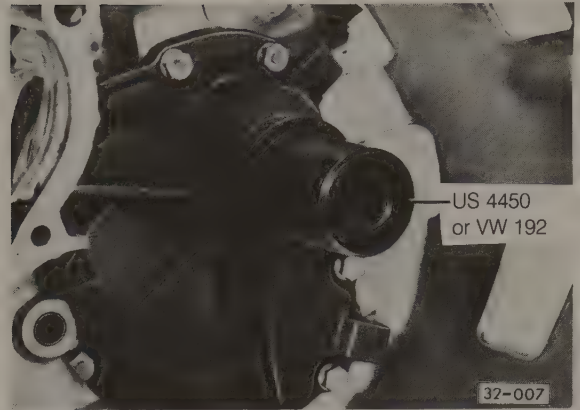
Fig. 5-7. Seal driver being used to install new torque converter seal onto one-way clutch support on final drive housing. Volkswagen special tool no. US 4450 or VW 192 shown. Use tool of approximate seal diameter to apply even installation pressure.
