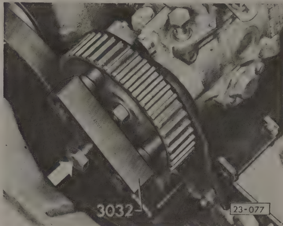
Fig. 5-14. Puller installed on fuel injection pump sprocket. Tension puller and tap bolt (arrow) to remove sprocket. Spacer between nut and puller screw prevents damage to pump shaft.
