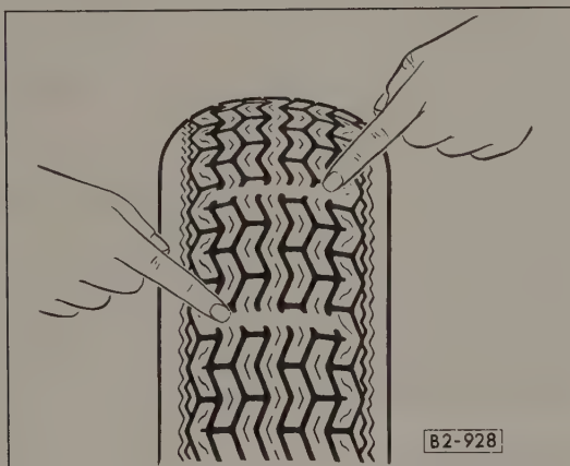
Fig. 3-1. Tread wear indicator bars showing on worn-out tire.
