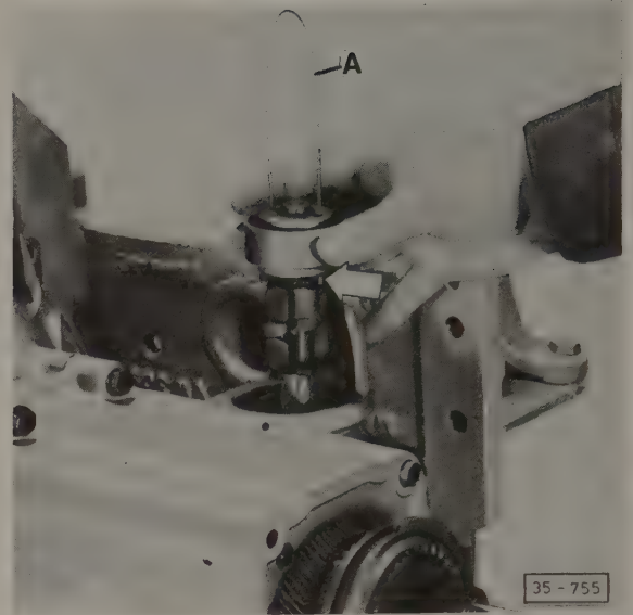
Fig. 6-9. Selector shaft (arrow) being installed. Bent coat hanger wire or welding rod (A) can be inserted as shown to keep shaft components from moving while engaging shift forks.
