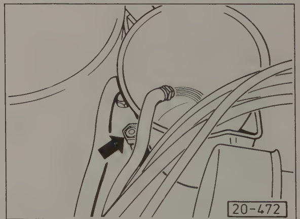
Fig. 4-7. Container being used to measure fuel delivery rate at CIS or CIS-E return line. Return line connection (arrow) is located near right (passenger side) front suspension strut tower.
