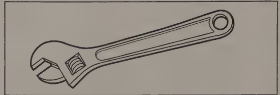
Fig. 4-7. Adjustable wrench is useful if used with care. Adjust for best possible fit. Use only when correct size wrench is not available.
