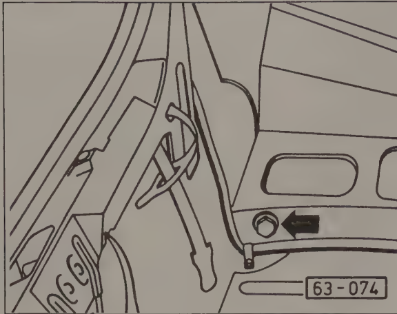
Fig. 6-19. Rear bumper mounting bolt (arrow) in luggage compartment. Remove bolts from left and right side.
