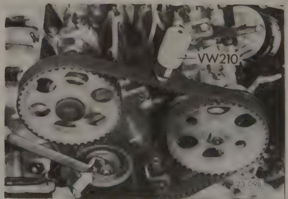
Fig. 5-13. Spanner wrench (arrow) being used to adjust belt tension. Volkswagen special tool no. VW210 is belt tension gauge.
