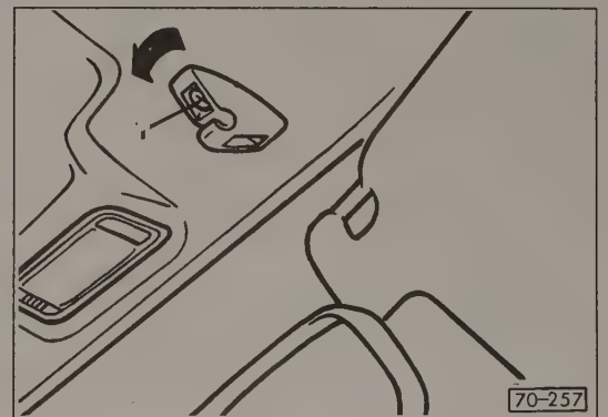
Fig. 4-48. Retaining clip mounting screw (1) to be removed, and direction clip is twisted (arrow).
