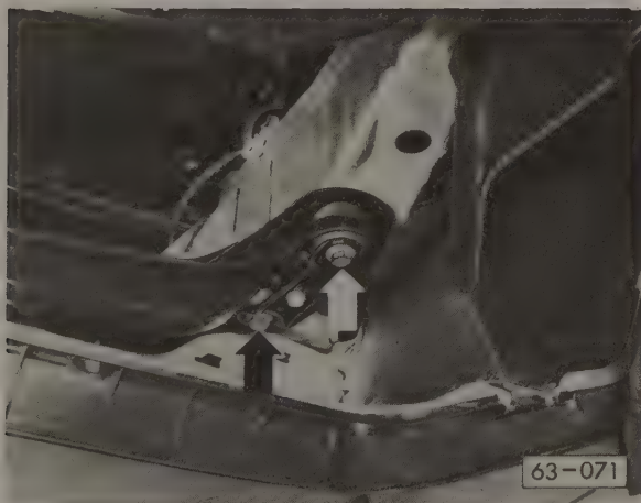
Fig. 6-16. Front bumper frame mounting bolts (arrows). Remove bolts from left and right side.
