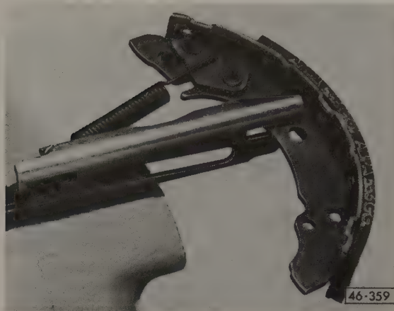
Fig. 6-5. Adjusting bar and tensioning spring being installed on brake shoe. Brake shoe and spring attachment are shown from behind.
